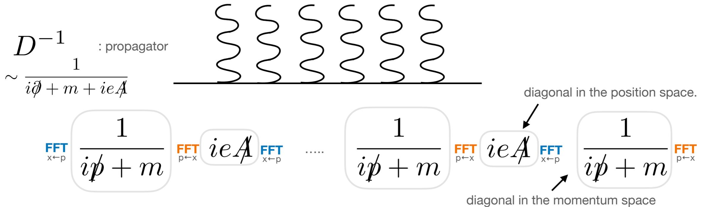
No integration or linear solver is necessary. **Sequence of multiplying diagonal matrices.**
